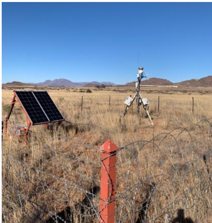
Figure 5 EDDY Covariant FLUX tower in the Karoo, South Africa (Source: Author)
